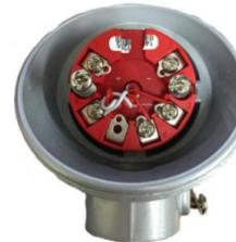
Terminal (1) wire = +24VDC from lower terminal block in LOGIX Axiom microcontroller.
